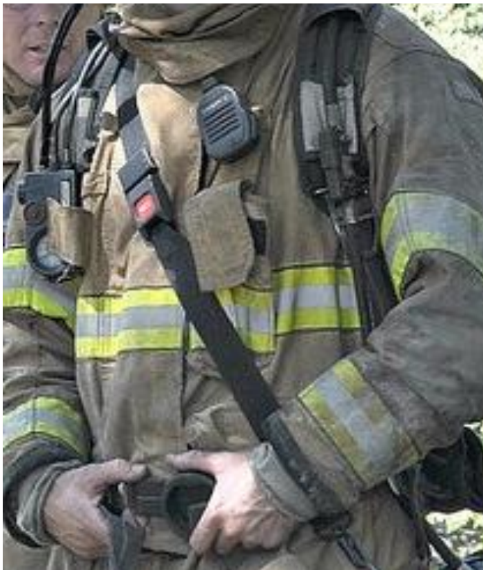
Figure 8 – Strap worn under the coat and protruding out of the natural gap between the buckle flap and collar flap. The majority of the RSM cord is protected.
